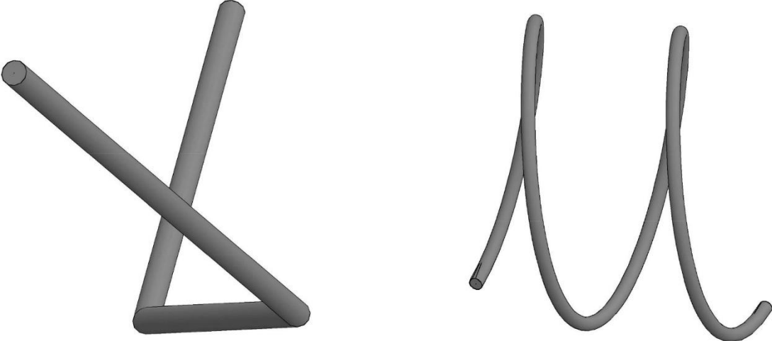
Figure 1. Proposed shapes of fiber reinforcement
