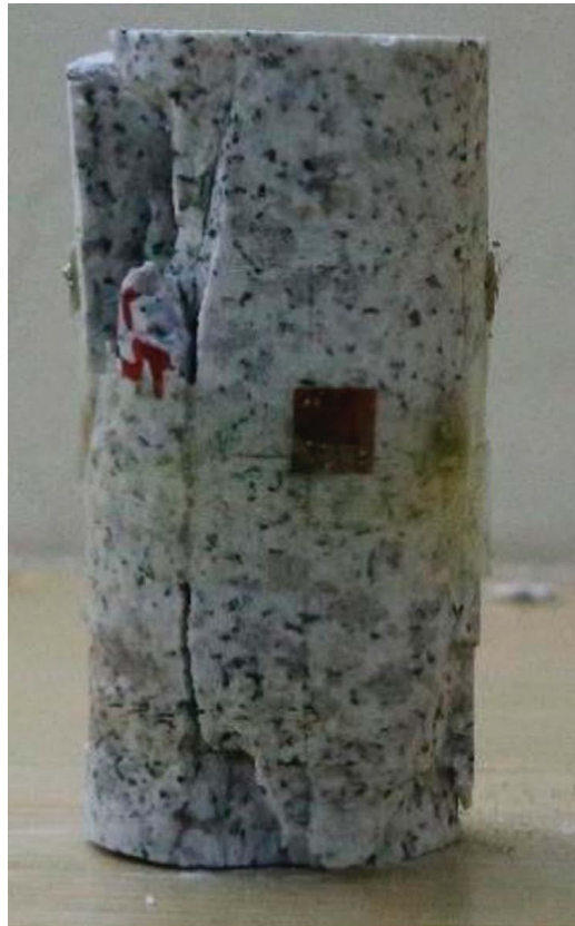
Figure 1. Appearance of a failed specimen
